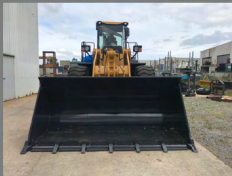
3.5m³ GP Bucket(Teeth/Secondary Cutting Edge)
