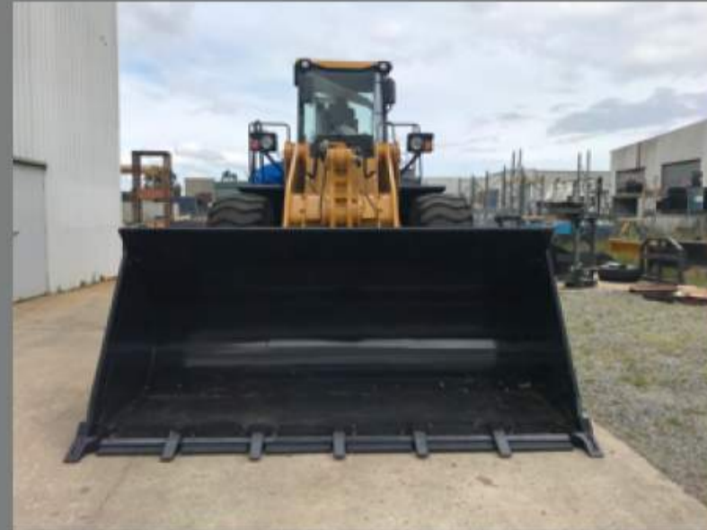
3.5m 3 GP Bucket (Teeth/Secondary Cutting Edge)
